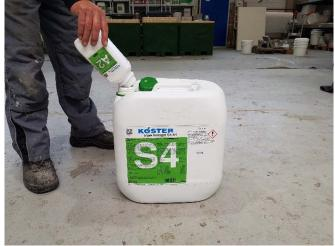
For the standard mixture, which gives a gel time of 40 seconds at  $70^{\circ}$ F, pour the entire B-component into the empty canister and fill with 20 kg of water to a height of 8.25 inches (can be marked in advance), seal, and mix by rocking for 30 seconds.The green canister can be cleaned and re-used.
